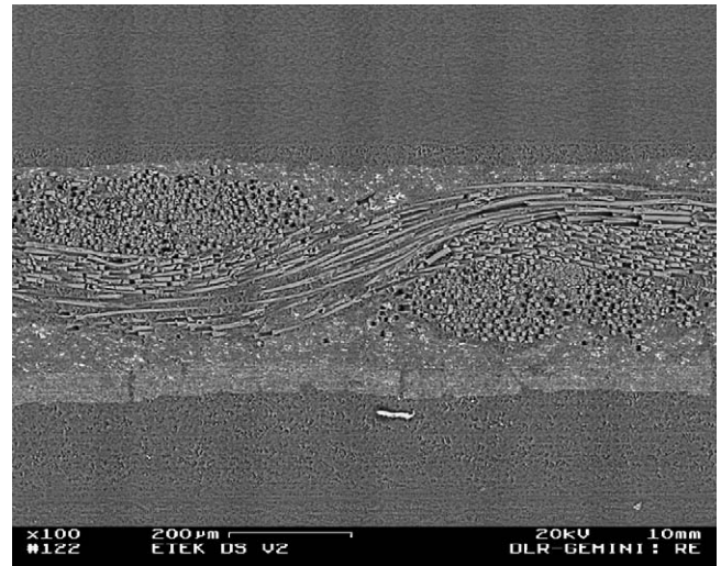
Fig. 5. SEM micrograph of an ELAT-DS electrode – cross-section – 100× magnification.
